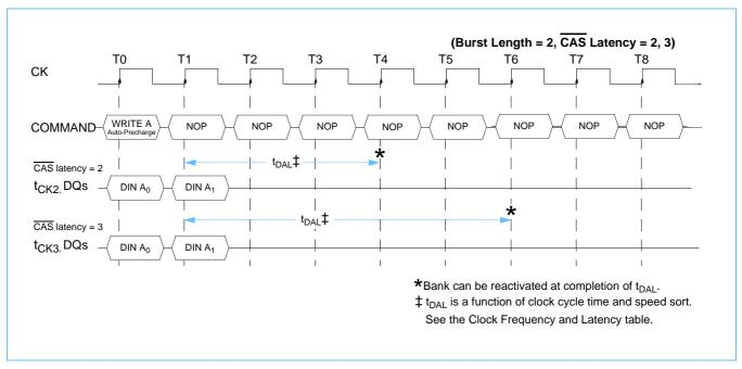
Similar to the Read Command, a Write Command with auto-precharge can not be interrupted by a command to the same bank. It can be interrupted by a Read or Write Command to a different bank, however. The interrupting command will terminate the write. The bank undergoing auto-precharge can not be reactivated until t<sub>DAL</sub> is satisfied.
